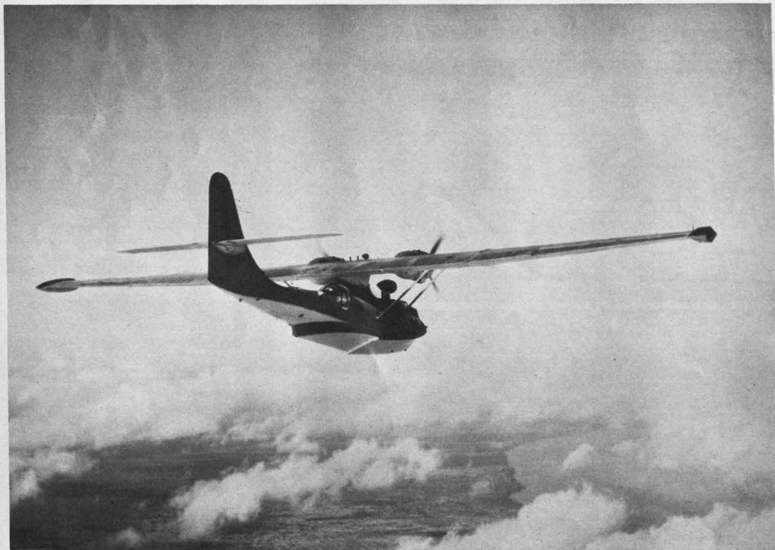
New Catalina, PBV-6A, has the tall tail of the PBN without incorporating latter's longer, more pointed nose. Prominent teardrop-shaped
